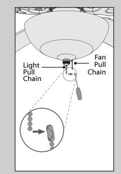
Thread the light pull chain through the hole in the finial and screw the finial onto the threaded rod. Connect the pull chain pendants to the short chains coming from the fan.
